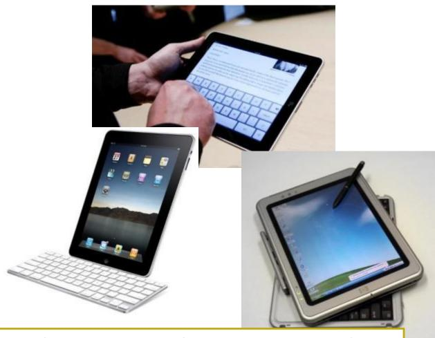
Tablet PC's (hybrids) and Tablet Computer's are fully functional computers with a touch screen, which allows input from a stylus, digital pen, or fingertips.
